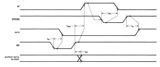
Figure 13. Strobed I/O Timing
